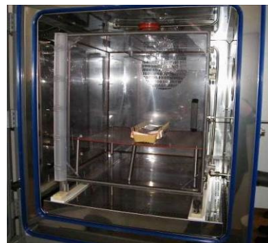
Laboratory test in chamber with mixed air pollution
