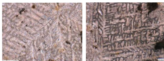
Morfologie povrchu Al55Zn povlaku po 10 a 15 letech expozice v Kopistech/Surface morphology of Al55Zn coating after 10 and 15 years of exposure at Kopisty
